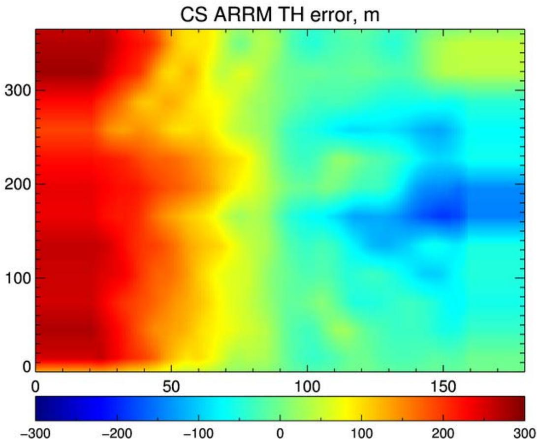
**Figure 1.** Altitude registration correction applied in V2.5 Level 2 processing as a function of event number and season. The X-axis scale shows event number along the orbit, and the Y-axis scale shows day of year. The Southern Hemisphere terminator crossing occurs at event 0. The color scale shows calculated tangent height error, ranging from -300 m [*blue*] to +300 m [*red*].
